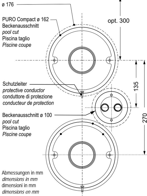
Abmessungen in mm
