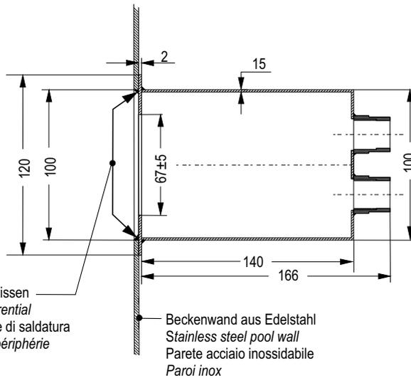
Abmessungen in mm / dimensions in mm
